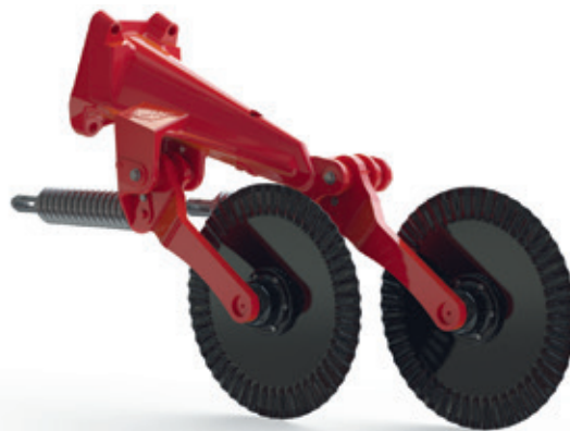
A 430 mm embossed disc cuts residues effectively and reduces soil projection.
