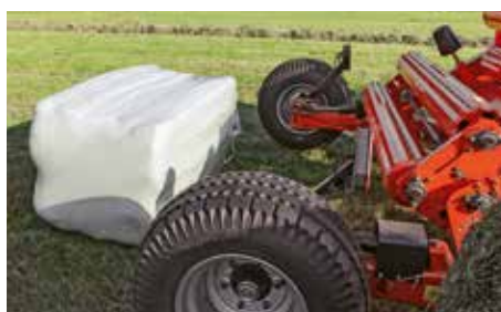
The low table height allows the bale to be gently tipped off to prevent film damage
