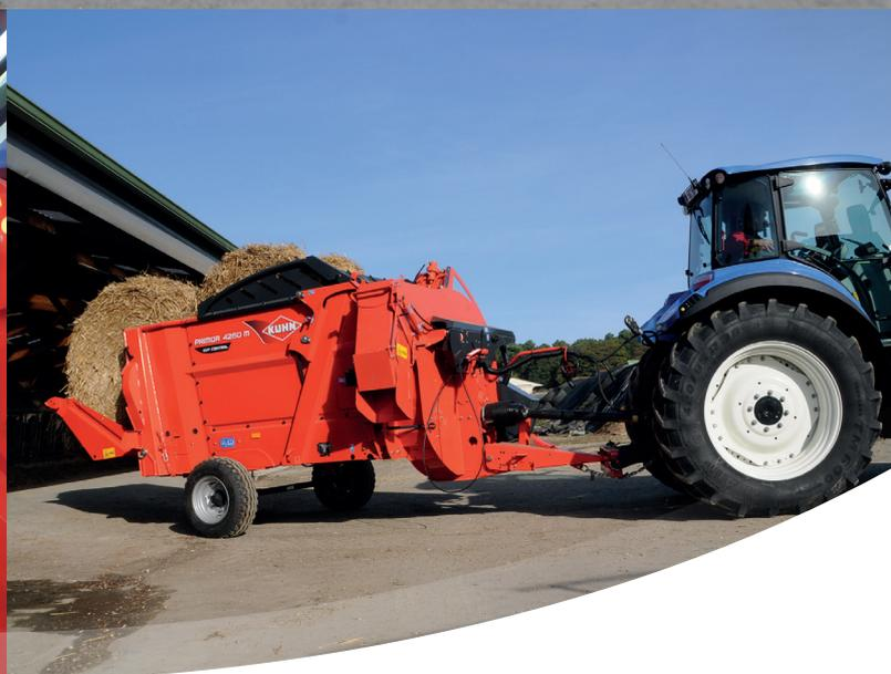
The PRIMOR 4260 M CUT CONTROL brings an additional feature to the straw blower and all-fodder feeder range: the **possibility of activating (or disabling) the chopping function**. The same machine can therefore be used to **put down short straw (cubicles) or long straw (bedded packs)** while retaining the capacity to deliver long-fibre fodder (such as hay or haylage).
