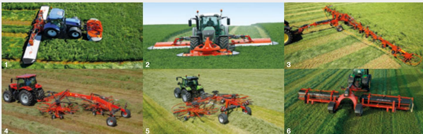
1. Triple disc mowers - 2. Triple disc mower conditioners - 3. Trailed gyro tedders with 13 and 17 m working width - 4. Semi-mounted twin-rotor gyro windrowers with side delivery - 5. Semi-mounted twin-rotor gyro windrowers with central delivery - 6. Conveyor belt windrowers
